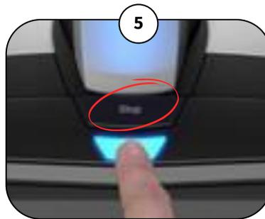
If the Scan Button is not lit in blue, press the Stop Button to activate scanner.
